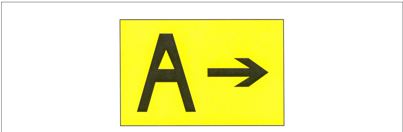
FIG 2-3-36 Direction Sign for Runway Exit
